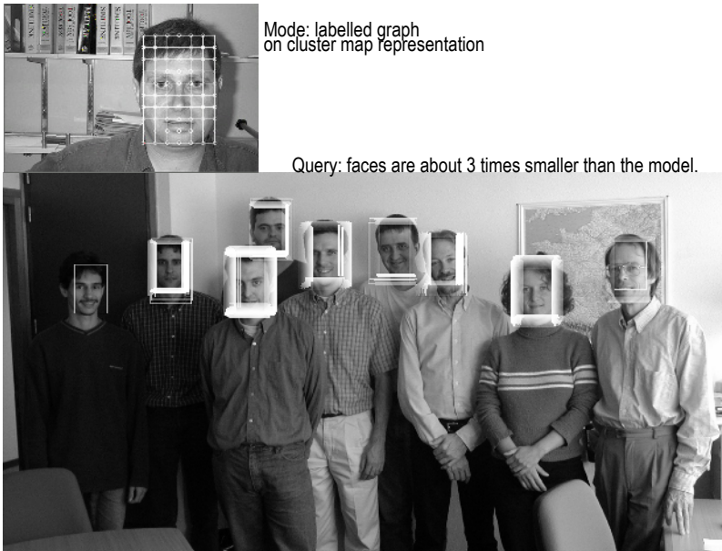
Fig. 6.7. Successful detection of faces in unconstrained images. The white rectangles mark the position and size of the graphs with lowest cost.
