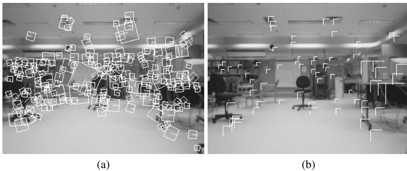
Fig. 17.2. (a) SIFT features found, with scale and orientation indicated by the size and orientation of the squares. (b) Stereo matching result, where horizontal and vertical lines indicate the horizontal and vertical disparities respectively (from [411]).
